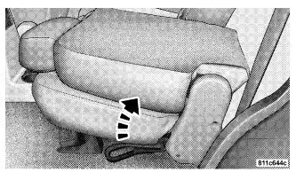
Raising the lever allows third row seat passengers to fold the seatbacks and release the latches when exiting the vehicle. Once the seatback is in a folded position continue raising the lever fully to release the cushion latches and tumble the seat. This folding and tumbling action provides easy access to the third row seat.
